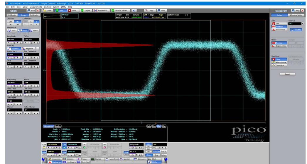
Behind the powerful measurement and display capabilities of the 9400 Series lies a fast, efficient data histogram capability. A powerful visualization and analysis tool in its own right, the histogram is a probability graph that shows the distribution of acquired data from a source within a user-definable window.
