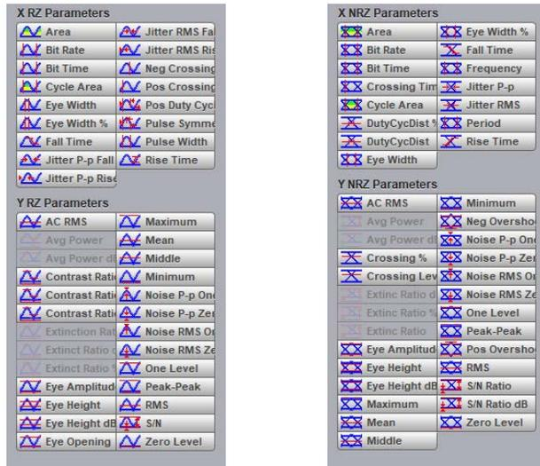
Eye diagram analysis can display data including: bit rate, period, crossing time, frequency, eye width, eye amplitude, mean, area and jitter RMS. Also shown on the graph are left and right RMS jitter markers. These measurements are selectable from within the Eye Diagram side menu and are listed on screen below the graph.
