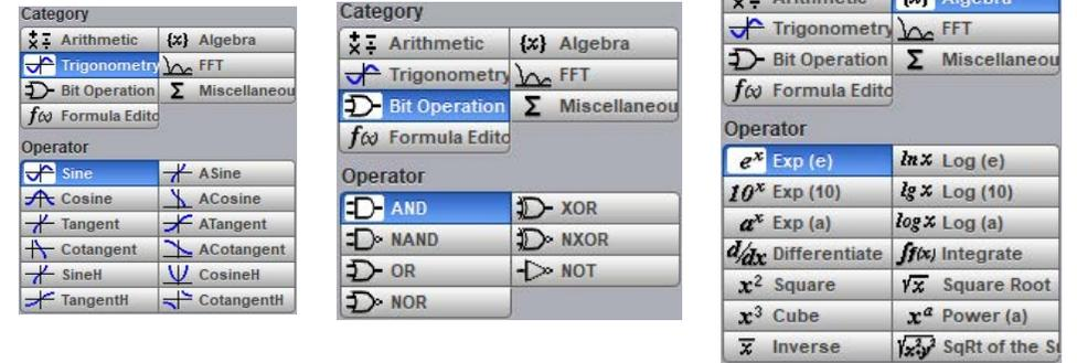
The PicoScope 9400 Series scopes support up to four simultaneous mathematical combinations or functional transformations of acquired waveforms.
