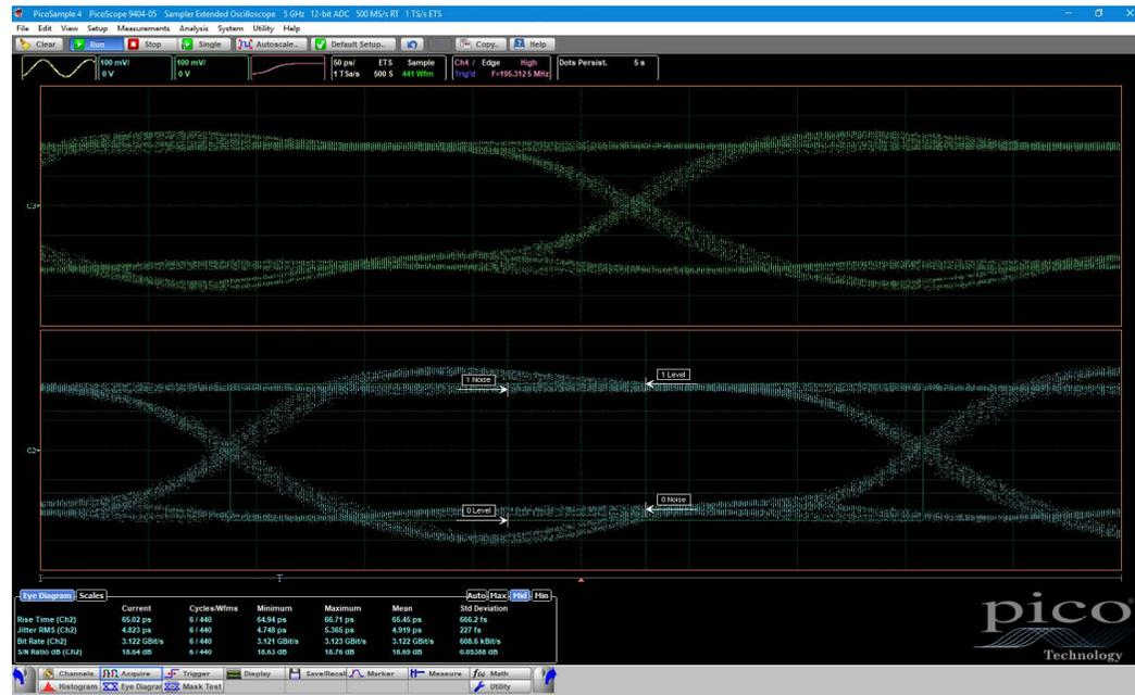
Eye-diagram analysis can be made even more powerful with the addition of mask testing, as described below.
