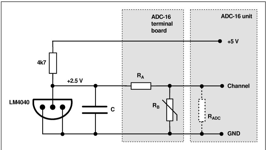
**Temperature sensor circuit with precision thermistor**
