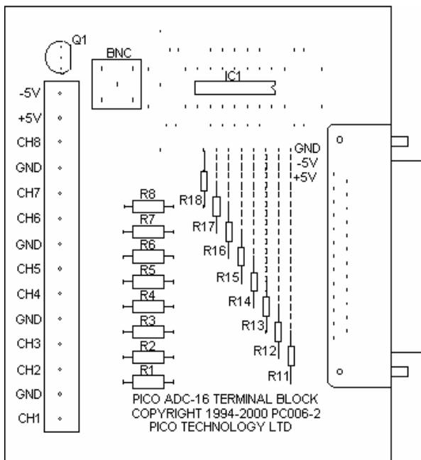
**Layout of ADC-16 Terminal Board**
