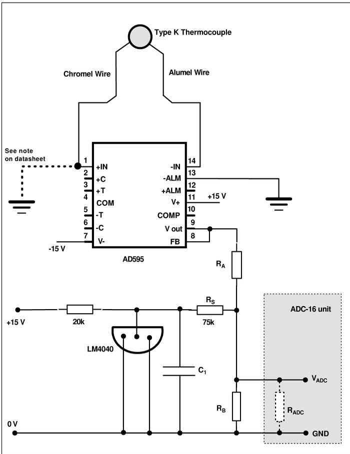
**Temperature sensor circuit with thermocouple and AD595**
