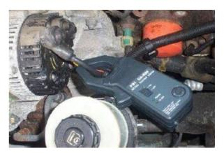
The clamp needs to be positioned around the wires on the back of the alternator. If this is not possible, then the clamp can be positioned at the battery positive cables. If possible, identify the wire that connects the alternator to the battery. If you clamping all positive wires at the battery, the clamp will read the difference between the total load and the charging current.
