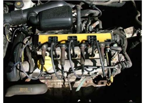
This system can only be tested if you have the same number of extension leads as coils within the cartridge coil-pack. The cartridge coil-pack is fitted directly over all the spark plugs and lifts off in one unit.
